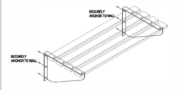
PLEASE ENSURE CENTRE OF SLATS LINE UP WITH PRE-DRILLED HOLES AS INDIGATED BELOW
