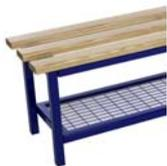
**Mesh Shoe Racks:** Constructed using a powder coated 30x30 formed angle support framework into which 50mm x 25mm mesh is fitted, simply bolts into the legs under the bench seat unit at 150mm centres from the floor.
